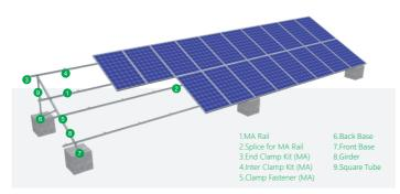
MRac Double-row Tripod Base-beam-free RMIV is derived from RM Il to meet different roof projects demands. Solar modules can be arranged with single or double rows of landscape or portrait orientation. Quick installation and stable structure are assured by the modular Patented design.
